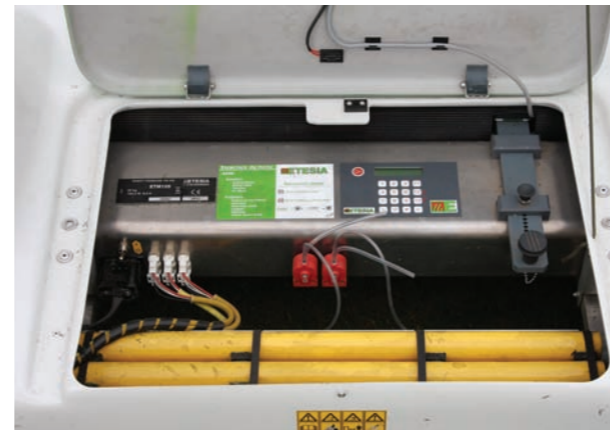
The keypad allows the user to enter a password to prevent the mower operating outside its fixed boundary. Key maintenance demand is to blow unit clean periodically with a compressor.
